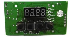
Pcb (Display) LED SLS-360 UV 36x1W Floor (LED-M9-V2.PCB)
